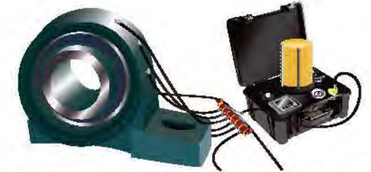
Direct lubrication of a bearing using combination of Easy Grease and hoseset.
